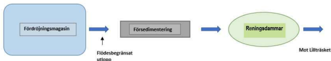
Figure 8-6 Schematic of the delay and clean up steps.
