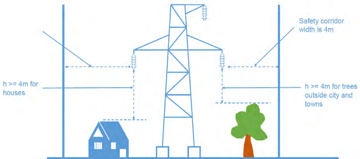
Figure 3.3 Safety Corridor Required for 110kv Transmission Lines
