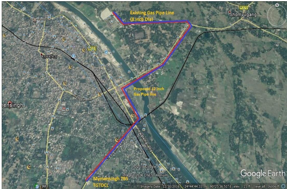
Figure 3.3: Gas supply pipe line existing 8” and proposed 12”
