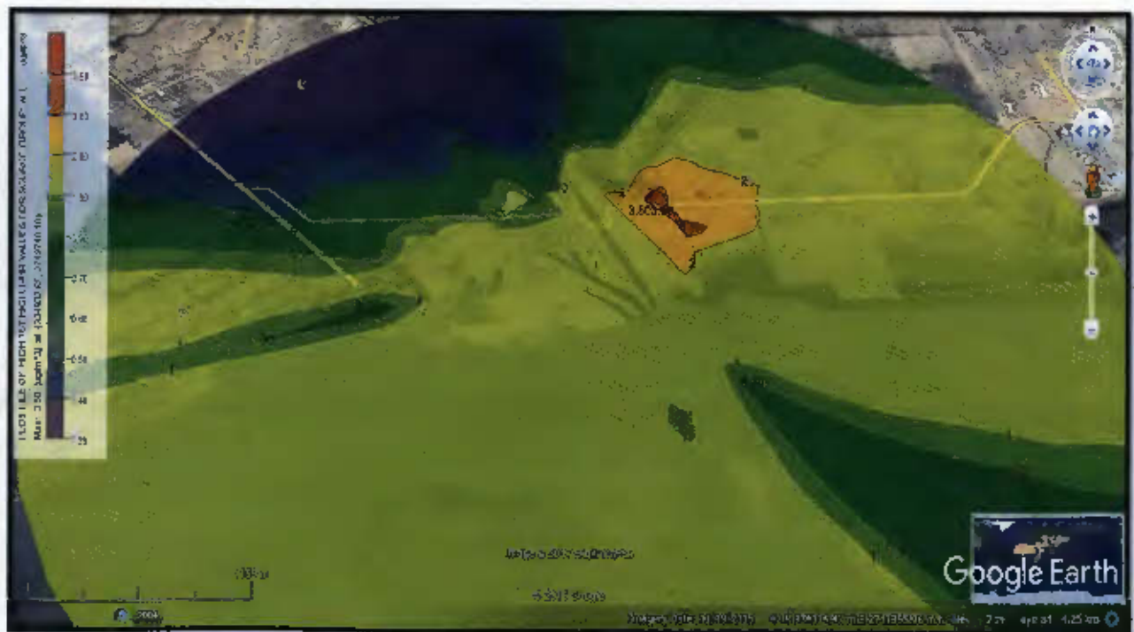
Figure 7: Spatial Dispersion of 1 st Highest Concentrations of CO for 1-hrly Averaged for Scenario-I
