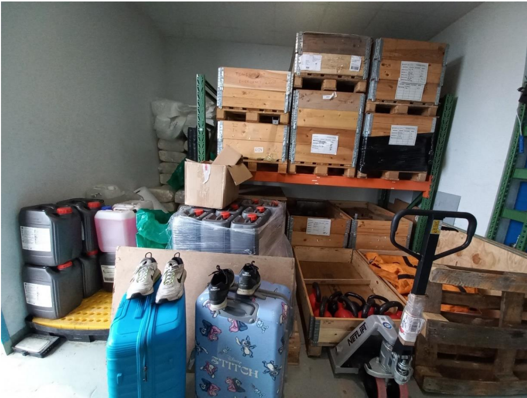
Chemicals Stored in Warehouse Room without Secondary Containment
