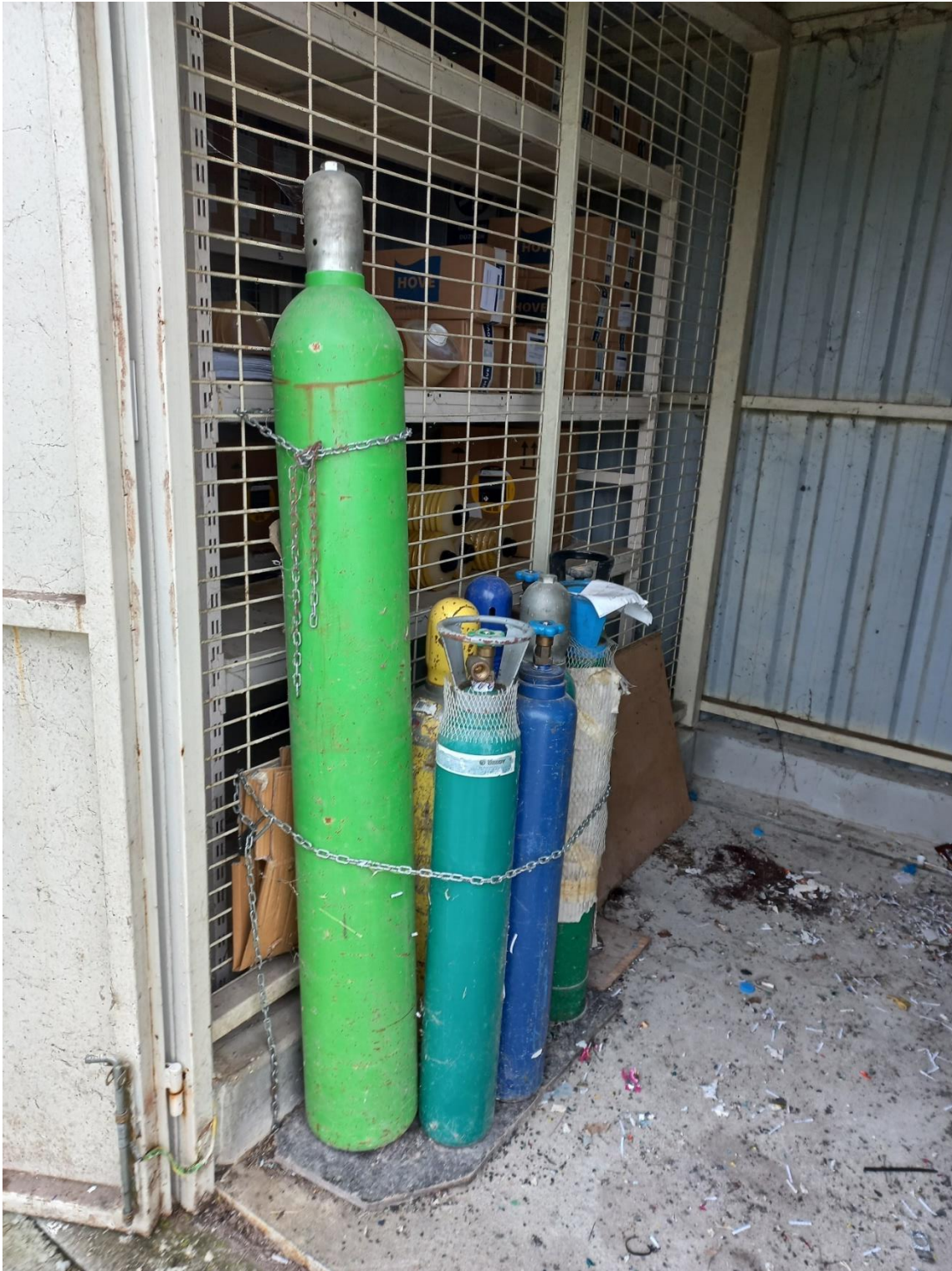
Storage of Gas Cylinders in Recyclable Waste Container
