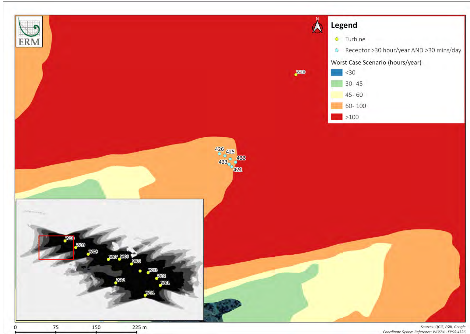
Figure 10.13 Map of Predicted shadow flicker at receivers no. 421 to 423, 425 and 426 (hours/year) – Worst Case Scenario
